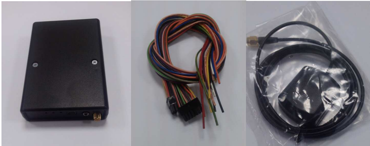
Figure2. FM Pro3 device, power and I/O cables and GPS/GLONASS antenna.
